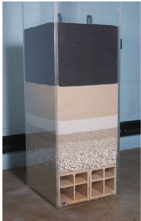
Water passes through charcoal, sand, and gravel layers in a water system's filtration tank.
